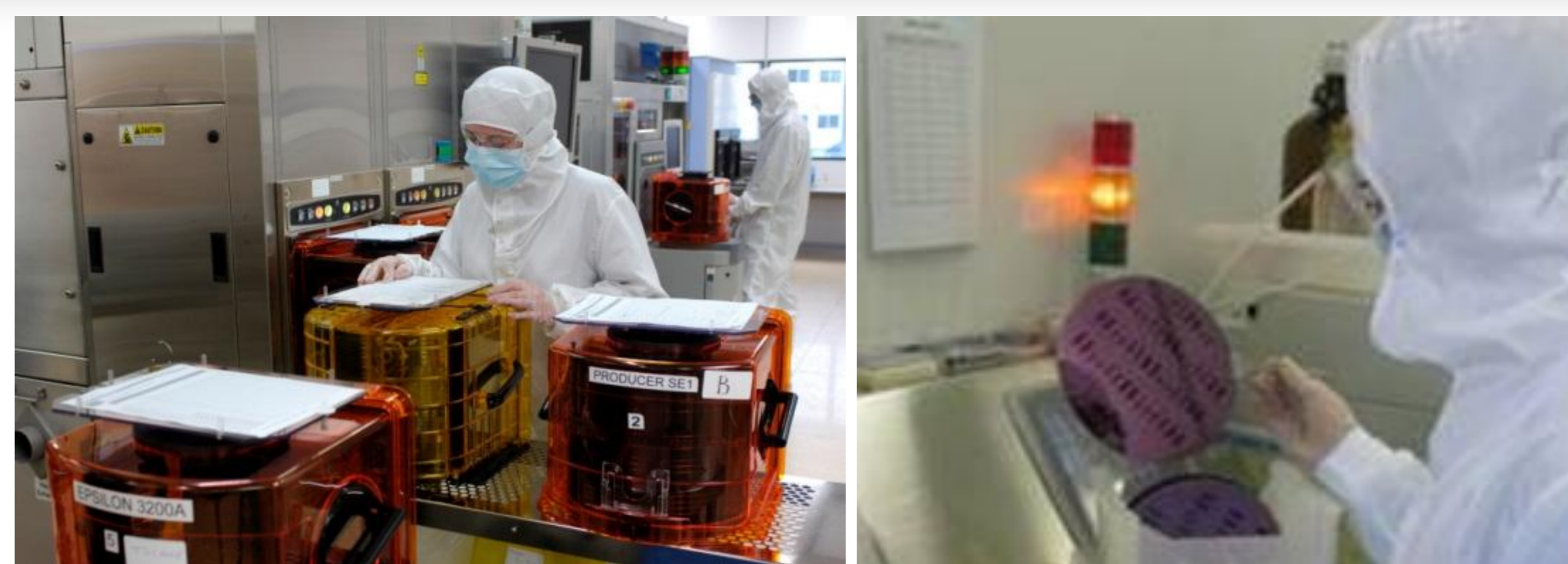
FOUP (Front Opening Unified Pod):
